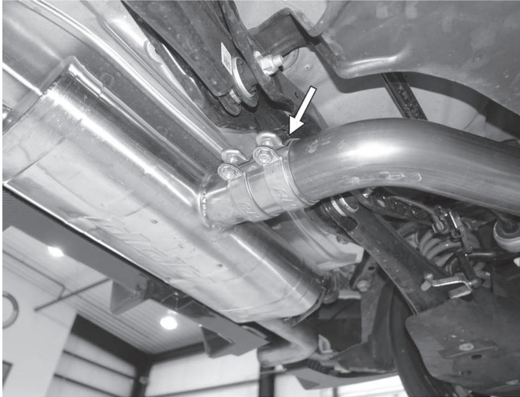
11) Connect the back of the APR bent pipe assembly to the APR rear muffler assembly with one of the supplied sleeve clamps. The clamp can be loosely tightened, but still needs to be adjusted.
