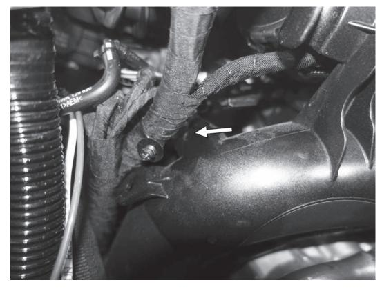
13) Pry off the clip holding the wiring harness to the top of the stock turbo outlet pipe.
