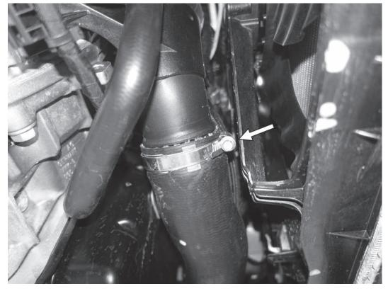
11) Loosen the 7mm clamp on the lower turbo outlet hose, and then separate the hose from the stock outlet pipe.
