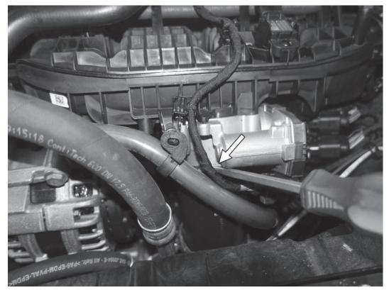
27) Using a pick tool or screwdriver, separate the hose from the throttle body by running the tool around the outside diameter of the throttle body inlet.
