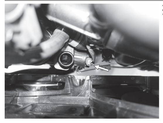
45) On the Golf R, reconnect the electrical connector to the diverter valve.
