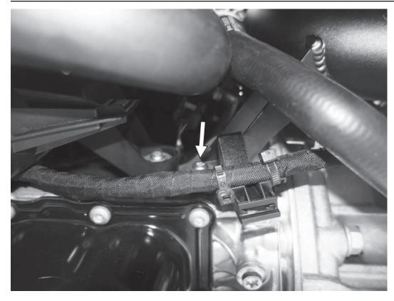
21) Install the factory T30 screw with the rubber grommet to the original stock pipe mounting point on the front of the engine. Torque the screw to 62 in-lbs (7Nm),
