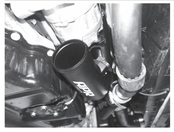
39) Place the APR front charge pipe assembly into the car from underneath.
