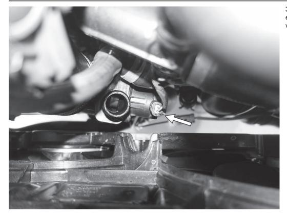
31) On the Golf R, disconnect the electrical connector to the diverter valve.
