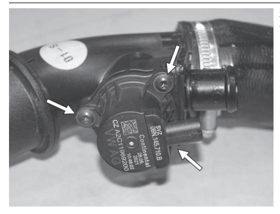
37) On the Golf R, remove the three T20 screws holding the diverter valve to the stock front charge pipe.
