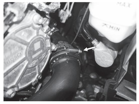
9) Loosen the 7mm hose clamp where the stock turbo outlet pipe connects to the turbo outlet hose.
