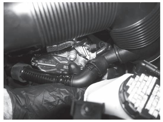
7) Lift up on the factory airbox to separate it from its mounting posts on the car. On the Golf R, disconnect the tube from the diverter valve to the back of the turbo inlet tube.
