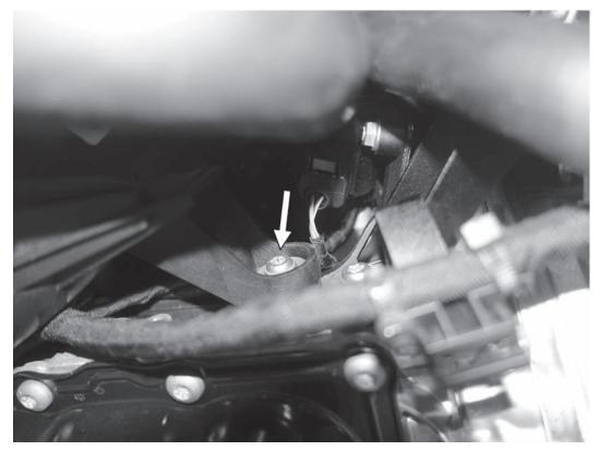
33) Loosen the T30 screw on the left side of the factory charge pipe. Pull the factory charge pipe down (with the upper hose to the throttle body attached) and remove it from the car.
