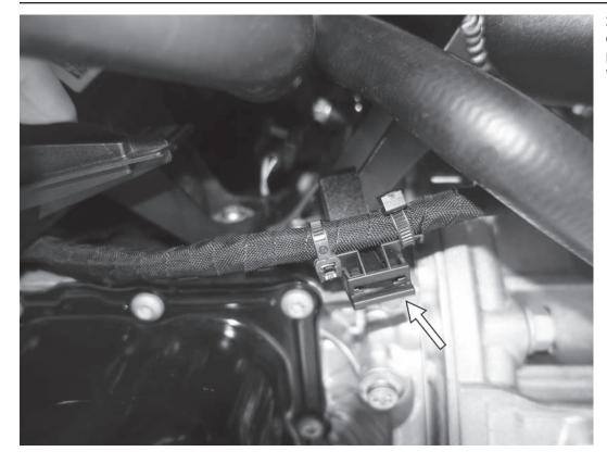
23) Install the wiring harness clip onto the mounting point on the APR pipe by simply pushing the clip onto the tab.
