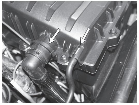
5) Disconnect the vacuum line from the right side of the factory airbox. If equipped, remove the secondary air hose from the side of the airbox by squeezing on both sides of the connector.
