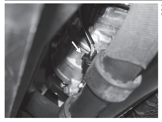
43) Reconnect the electrical connector from the wiring harness to the MAP sensor.
