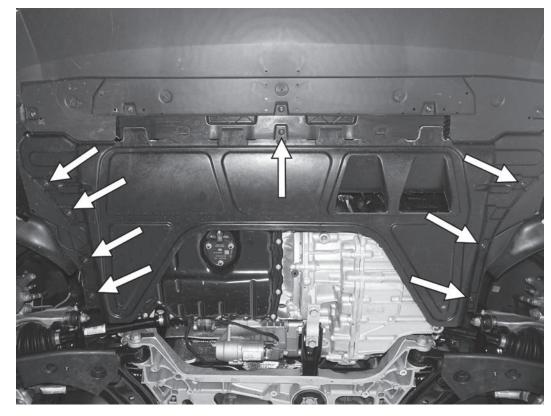
51) Reinstall the factory belly pan on the car, making sure the tabs of the belly pan connect to the bottom of the bumper cover as they originally did. Secure the belly pan with the eight T25 screws.
