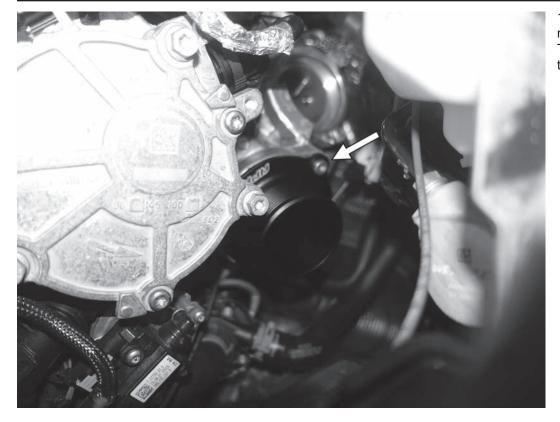
17) On the GTI, install the APR turbo muffler delete with the three original T30 screws, and then tighten the three T30 screws to 9Nm (80in-lbs).
