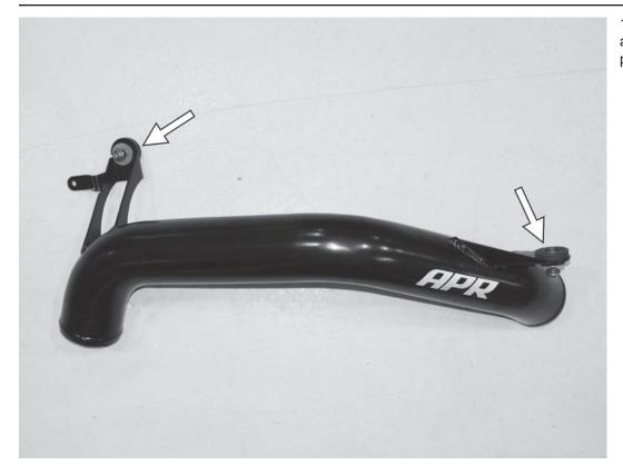
19) Install the two rubber grommets and screws onto the APR turbo outlet pipe as shown.
