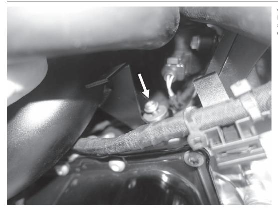
41) Secure the APR intercooler pipe by installing the T30 screw on the left side of the pipe. Torque the screw to 62 in-lbs (7Nm).
