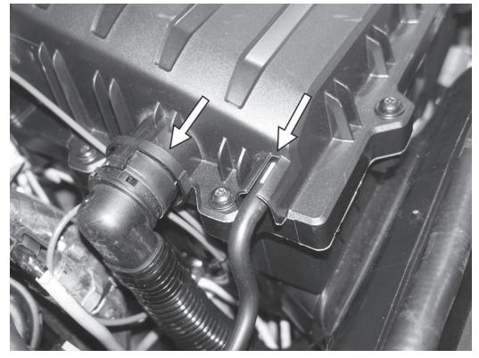
49) Reconnect the vacuum line to the side of the airbox. If equipped, install the secondary air hose to the side of the airbox.
