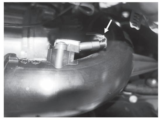
29) On the lower side of the factory charge pipe on the front of the engine, disconnect the electrical connector to the factory MAP sensor. Pull the small tab out and away from the sensor, and then squeeze on the connector to release it.
