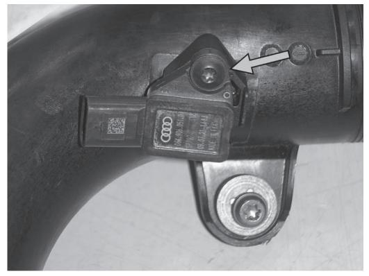
35) Loosen and remove the T20 screw holding the factory MAP sensor to the factory charge pipe. After noting the direction of the MAP sensor electrical connector and how it is oriented in the pipe, remove the MAP sensor from the pipe.
