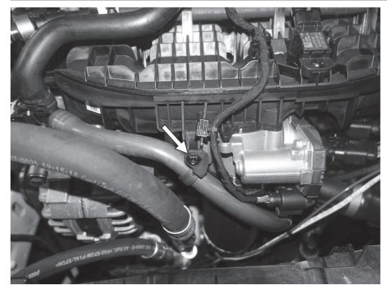
25) Remove the T30 screw holding the hose to the front of the intake manifold, by the throttle body.
