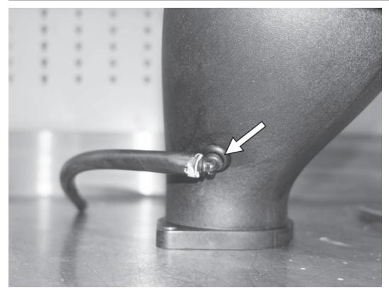
13) Install the 90° barbed fitting into the grommet on the APR filter adapter, and then install the supplied rubber hose onto the barbed fitting.
