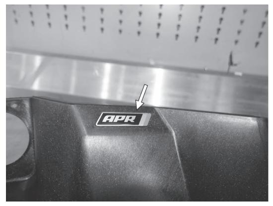
7) After removing the adhesive backing, place the APR logo in the recessed location on the top of the back of the APR heat shield.
